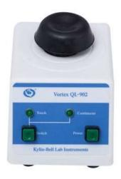
It has a ultra small design with new appearance. The QL-902 is molded by ABS engineering plastics without any spray of paint. The body is acid, alkalis, and corrosion resistant. It provides point oscillation and continuous function with the natural wear – resistant rubber bowl, which will accelerate the experiment. The cast iron stable base will not move or rotate. It is suitable for quick mixing of different sample cells with 0.5 ml to 50 ml.
